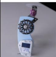
Positive yarn tension feeder system-For stable and quicker spandex feeding.
